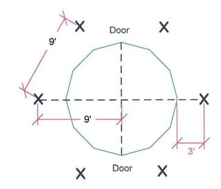
come in two lengths, one slightly greater than the other. Select one of the three longer spokes. Since it's about six feet long, its midpoint will be at three feet, and that's how far you want the stake to be from the ground cloth. You want to drive this stake into the ground at least a 45° angle to the ground, for maximum leverage and holding power. Move your marking spoke to the next station, and repeat the process. This should give you six stakes spaced evenly around the center of the tent.
