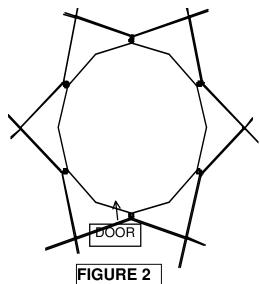
If your sidewalls have zippers, the first sidewall starts at the point where the guy lines come down at the door area. Proceed counterclockwise inside the tent, hanging the hooks off the D-rings next to the spokes. Hang the second sidewall, bearing in mind that there is no overlap.
